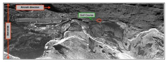
Examination of the image confirmed that the test piece had been detected, indicated by a bright white return on the radar image. A second radar return was seen on the image in the vicinity of the test piece. The cause of this return was not known and when the team returned to the site, we discovered metallic fencing wire buried under the snow.
