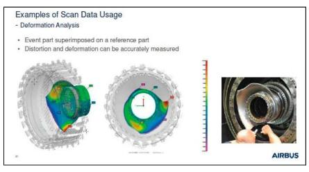
Advantages of the 3D scanning is that it provides an accurate record of parts as they were recovered and before any disassembly or destructive testing. The data can be made available to all parties of the investigation so that analysis can begin simultaneously. The data can be imported into Catia or viewed as a 3D pdf model.
