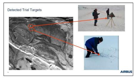
This demonstrated that the technology is fundamentally capable of detecting metallic objects even when buried under snow.
