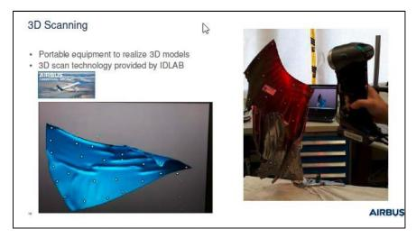
The scanned data allowed an assessment of which parts had been recovered and which remain on the ice sheet. A 3D reconstruction was produced which allowed an insight of how the engine event may have unfolded.
