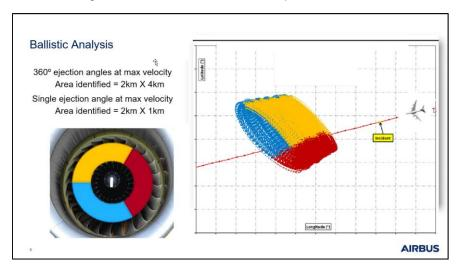
The ongoing investigation established the fragment ejection angle and ejection speed. This allowed the area to be refined to 1km x 2km. The parameters of the liberated parts has an effect on the ballistic analysis. Smaller heavier parts will be projected forward of the event point while lighter, larger parts which have aerodynamic drag will be carried rearwards of the event point in the direction of the wind.
