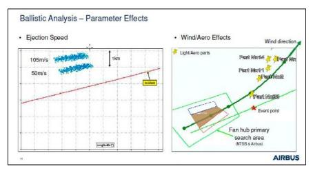
The fan hub primary search area shown above was identified using both Ariane and NTSB ballistic analyses, which were largely consistent.
