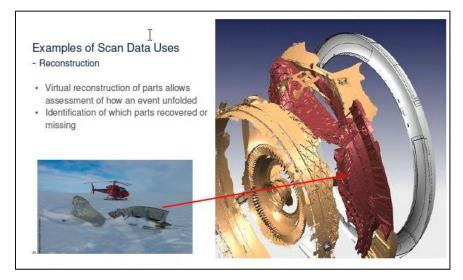
Further, 3D models can be overlaid to reference data such as Catia models or scans of reference parts so that an analysis can made on how a part had distorted or deformed.
